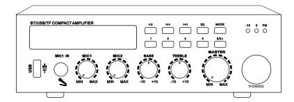
This Compact USB/TF/BT Mixing Amplifier provides 60 watts of output power with with bluetooth, intergral USB audio player power, and 5 inputs including 3 balanced MIC (MIC1 has another port of 6.35mm jack on front panel), 2 unbalanced AUX, each one has individual volume control.
