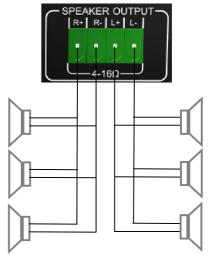
(The short circuit of the terminals between the left and right channels shall not be allowed; the output of the power amplifier is the bridging output; the negative output shall not be connected to the enclosure or grounded)
