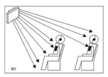
The Direction and Sensitivity of IR Receiver (Fig.1)
